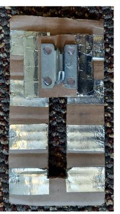
As the sliding piece moves, it makes and breaks connections between legs that are <u>next to each other</u> (not across from each other) - the photo shows a model of how the inside works!
